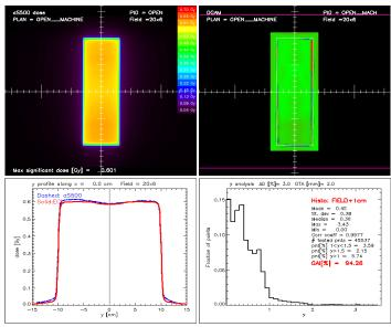
**Wedge field evaluation** - mechanical and dynamic wedge calculation vs. measurement
