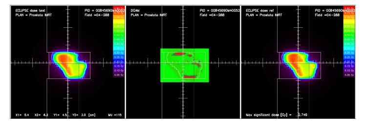
2. Example of calculation algorithm influence - comparison of the AAA algorithm results (right) and PBC algorithm (left).
