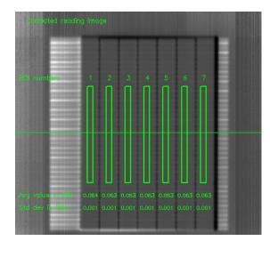
2. Precise MLC positioning during gantry rotation. Picket fence test is performed using sliding window technique while gantry rotates over 330 degrees. Epiqa allows visual and qualitative analysis of the performance of each leaf pair separately.
