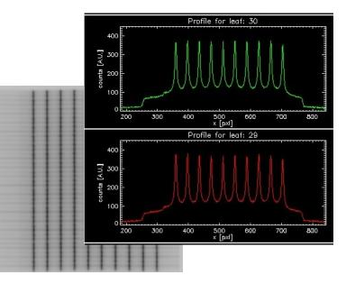
**3.** Accurate control of MLC leaf speed during gantry rotation for 4 different leaf speeds. Results of this tests are influenced by correct performance of MLC motions but also by gantry speed and correct dose rate. Each of the 4 strips are irradiated for 30 MU with the combination of different leaf speed, dose rate and gantry speed. ROI is analyzed for its average value and standard deviation.
